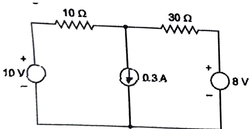
(c) Use superposition theorem to find the voltage  $V$  in Fig below
