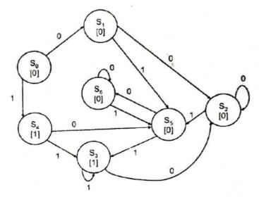
Q.3 A Mealy finite state machine has one input (X) and one output (Z). After each reset, an output Z=I occurs every time an input sequence of 000 or 101 is observed and an output of Z=O occurs whenever any other input sequence is observed. (Sequences may overlap.)
