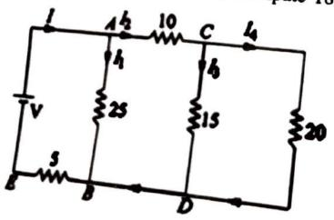
(b) Determine current in each branch of the network shown in figure using Nodal Analysis. (7)
