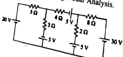
(a) With the help of Norton Theorem, find V<sub>0</sub> in the circuit shown in figure. All resistances are in ohms.
