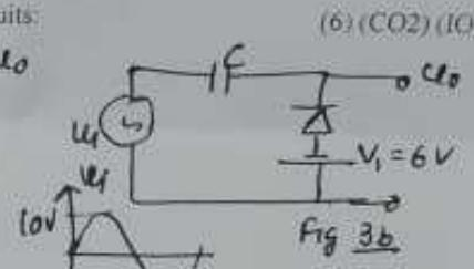
Q4. For the given circuit find (i) dc output voltage in each case. (ii) PIV for each case. Assume diodes are ideal. (4) (CO2) (LOCQ)
